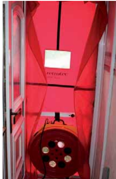
Blower door airtightness test. Source: MosArt Architecture
