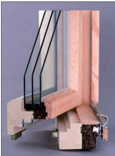
Externally insulated window frame reducing heat loss Source: Optiwin GmbH
