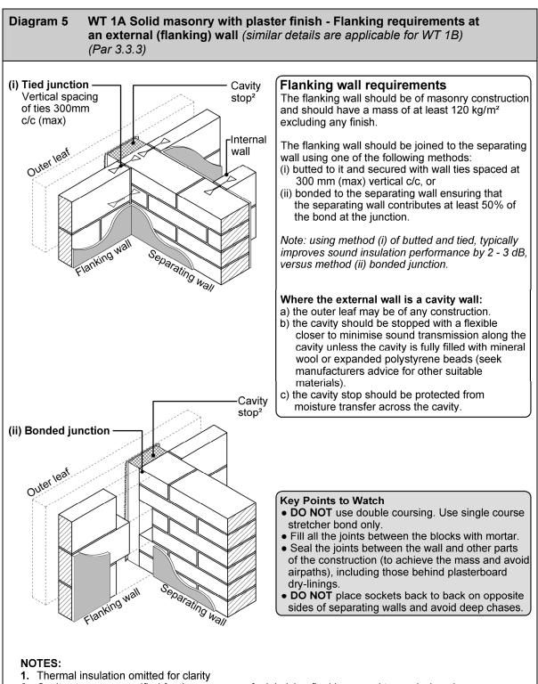
Cavity stops are specified for the purposes of minimising flanking sound transmission along the cavity. A cavity stop may also be required to act as a cavity barrier for the purposes of compliance with Part B - Fire Safety, see TGD B.
