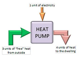
Figure 1: Heat Pump Coefficient of Performance (COP)
