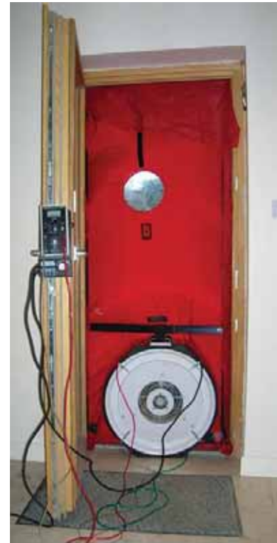
No more than 0.6 air changes/hour at 50 Pascal pressure should be observed in accordance with the Passivhaus Standard. This should be checked for compliance with a blower-door test which will immediately highlight leaky areas. Airtightness can be achieved through the use of membranes, roofing felts and plasters combined with sealants and vapour diffusion resistant materials.
