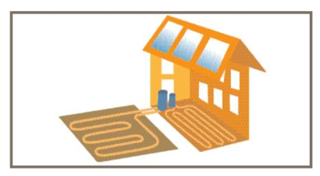
on whether the ambient air is colder or warmer than the soil. In winter, the heat pump removes the heat from the fluid, upgrades it to a higher temperature for use in the building, typically in under-floor heating.
