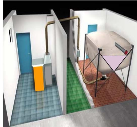
Boilers are available with varying levels of automatic cleaning and ash removal, from fully automatic to fully manual and many levels in between. Whatever wood boiler you choose, it is important that the recommended cleaning and ash removal schedules are strictly adhered to. If not, then over time the operational efficiency of the boiler will be significantly compromised.
