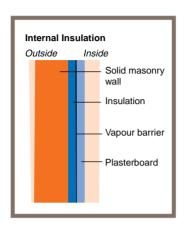
vapour barrier may be fixed to the wall. The work is quite labour-intensive, involving the repositioning of skirting boards, any electrical sockets or switches and other wall attachments.
