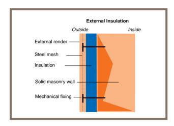
It is worth asking the installer if the proposed external insulation system has independent certification, for example from the Irish Agrément Board or equivalent. Such certification means that the system has been tested by an independent body and found fit for the purpose for which it is intended.
