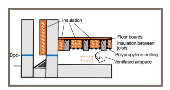
In all cases, the designer/builder should try to minimise penetration of the insulation by pipework and wiring, and to keep heating pipework above the insulation in order that heat loss from the pipework contributes to heating the room above.
