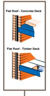
If you have an existing flat roof, insulation can be increased externally with extruded polystyrene or foamed glass, or internally with an insulated lining board such as mineral fibre or polyurethane foambacked plaster-board.
