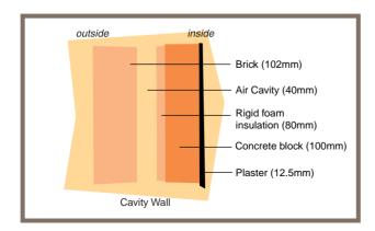
To calculate the U-value of this wall we must first calculate the combined thermal resistance of the various layers to account for heat lost due to conduction.
