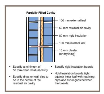
When full-fill cavity insulation is being used it is essential that such walls are designed and constructed to incorporate the normal precautions to prevent moisture penetration. Insulation thickness should remain constant and should any change in vertical thickness occur, a horizontal damp-proof cavity tray should separate each thickness change.
