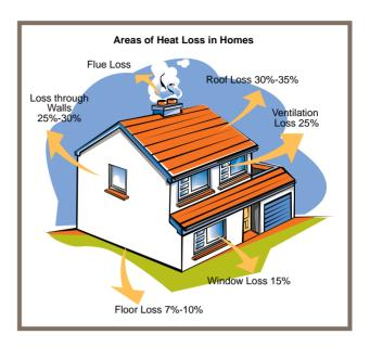
Since increasing insulation thickness does not produce a prorata reduction in U-value, there comes a point where the economic return on additional insulation for any one element will be virtually nil.
