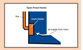
Building Regulations require that permanent ventilation openings are provided in such rooms. Provided adequate vents exist and are not blocked off, the room's windows may be draught-sealed. If in doubt, seek professional advice.
