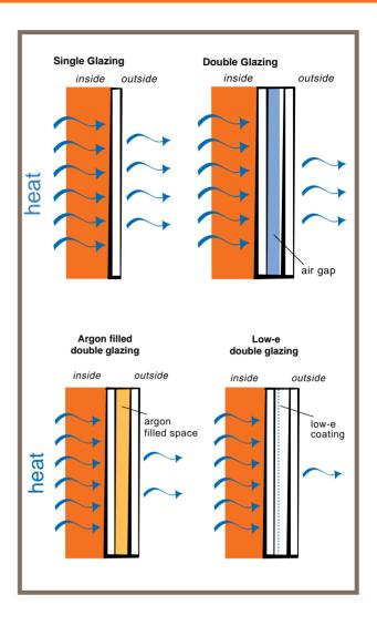
This will generally cost between 10-15% more than standard double glazing but is very energy-efficient. In both Denmark and Germany this form of glazing is fast becoming the standard installed in all buildings and it is possible that in Ireland it will also become the norm in the not too distant future. Other combinations of glazing systems include lowegas-filled double glazing or triple glazing.
