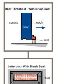
Letterboxes with just one inward-opening flap will tend to admit draughts, particularly when the wind is blowing directly on the front door. Brush seals are commonly used to reduce draughts through this type of letterbox.
