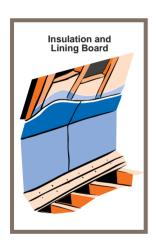
Lining boards can have integral insulation backings, such as glass-fibre-backed insulated plaster and urethane-foambacked insulated plasterboard, often lined with aluminium foil.
