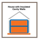
0.025 to 0.04 W/m K). Insulating the cavity with such materials will typically reduce heat loss through the wall to one-third of its original value. Such cavity insulation materials are generally water-repellent and rot-proof and some are non-combustible.
