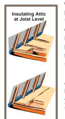
ceiling joists. This method requires a professional contractor. Be careful not to compress fibreglass insulation, otherwise it will lose part of its insulating value. So if boarding is to be put down in some areas of the attic for storage, it should not compress the insulation.
