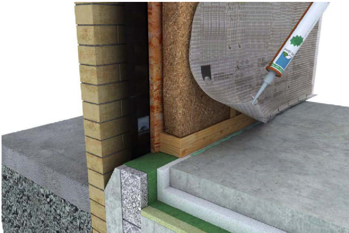
Figure 5 Bonding an air-tight membrane to the concrete floor slab
